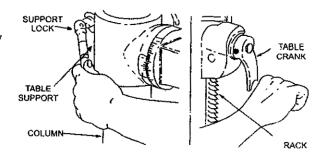
Remove protective covering from table and discard. Place table in table support and tinghten table lock (located under table)by hand.
