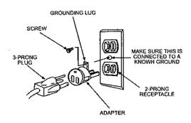
**NOTE**: The adapter illstrated is for use only if you already have a properly gronded 2-prong receptacle. Adapter is not allowed in Canada by the canadian Electrical Code.
