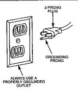
This power tool is equipped with a 3-conductor cord and grounding type plug, approved by Underwriters Laboratories and the Canadian Standards Association. The ground conductor has a green jacket and is attached to the tool housing at one end and to the ground prong in the attachment plug at the other end. This plug requires a mating 3- conductor grounded type outlet as shown.
