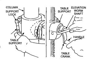
8. Check column collar for proper adjustment. Collar should not be angledon the column and it should be positioned so rack will slide freely in collar when table is rotated 360° around column table. If re - adjusted, only tighten set screw enough to keep collar in place.
